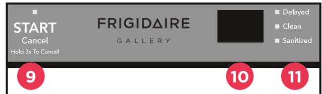
9. START CANCEL to start or cancel cycle. Door must be closed within 4 seconds of pressing START to start a cycle.
